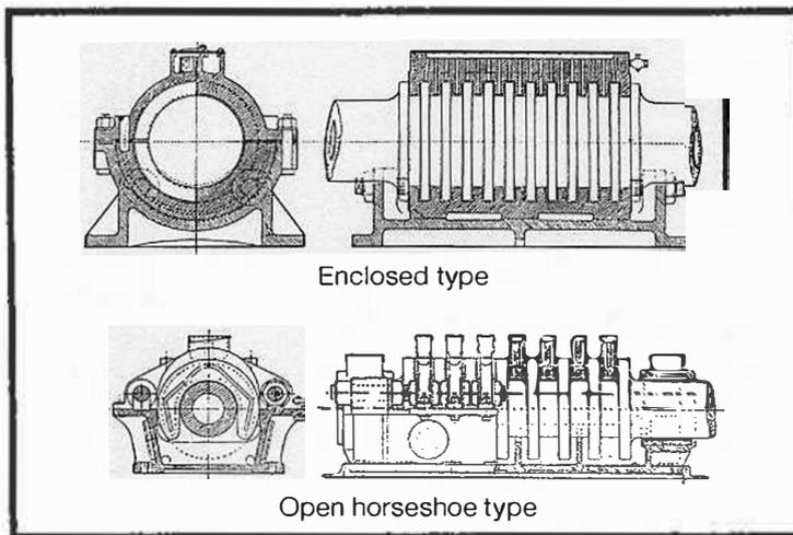
**Fig 2: Multi-collar thrust blocks**
