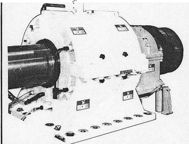
Fig 6: HMS *Invincible*; thrust block on test bed in maker's factory, 1979
