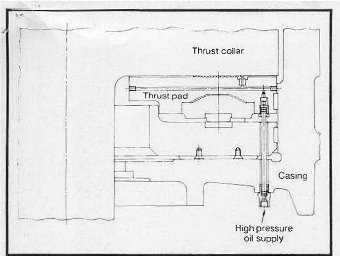
**Fig 9: High pressure jacking and three piece thrust pad construction**
