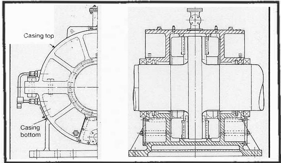
Fig 7: Concentric cylinder casing structure of a modern naval thrust bearing
