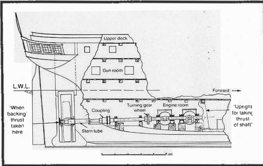
**Fig 1: Screw steamship HMS Ajax 1848; method of receiving thrust of screw propeller in either direction**
