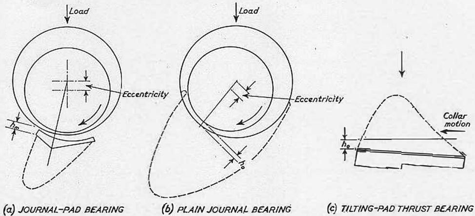
FIG. 1—Film thickness and pressure distribution in hydrodynamically-lubricated bearings
