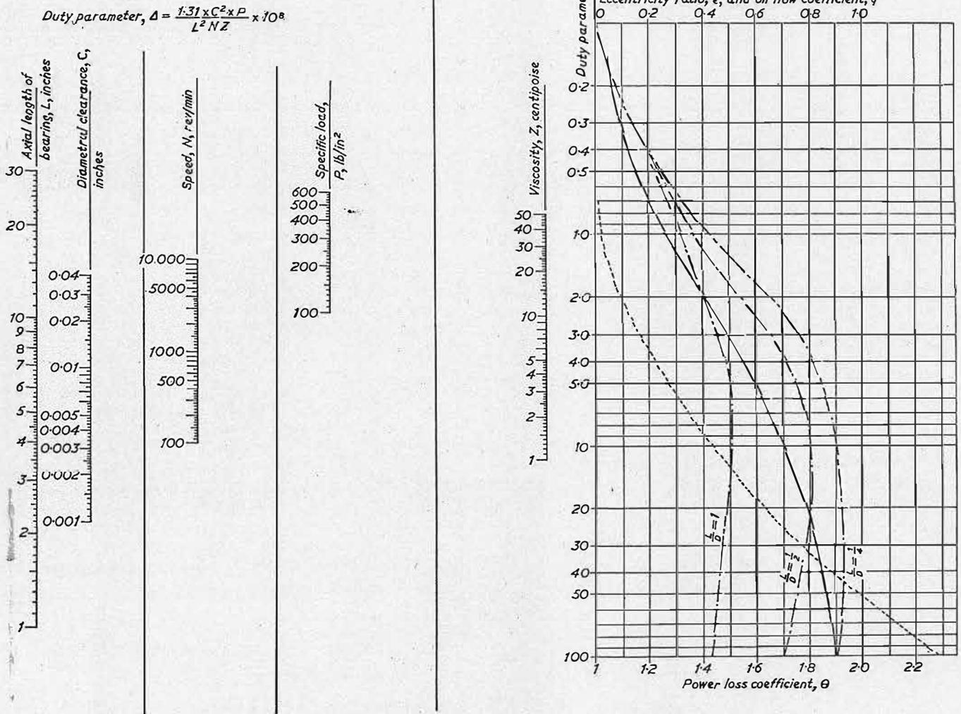
FIG. 2—Nomogram for eccentricity ratio, power loss coefficient and oil flow coefficient
