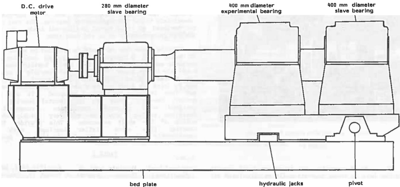
**SCHEMATIC DIAGRAM OF THE EXPERIMENTAL ARRANGEMENT**
