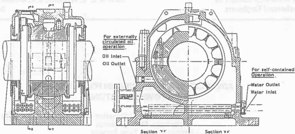
400 mm SHAFT DIAMETER EXPERIMENTAL THRUST AND JOURNAL BEARING
