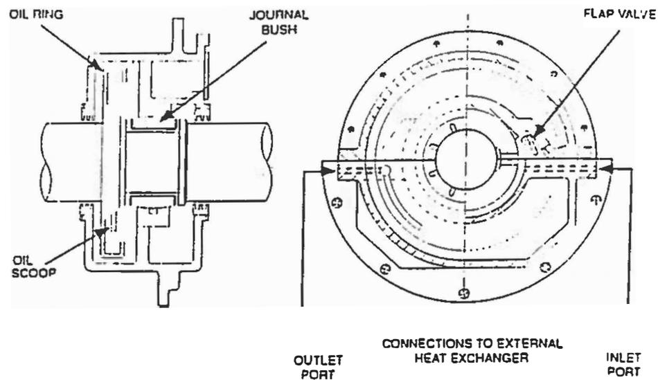
**Figure 2. Test Bearing**
