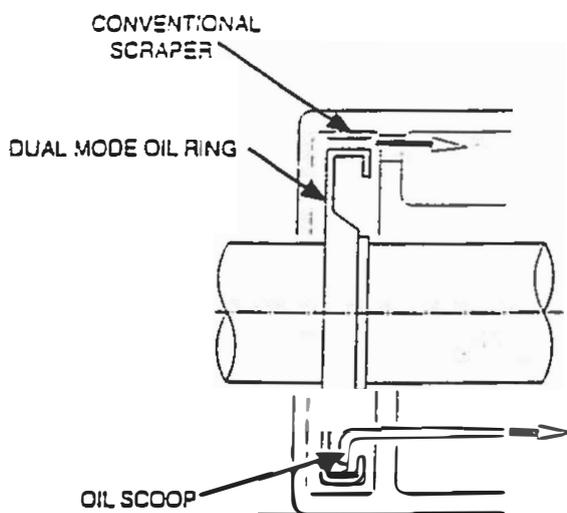
**Figure 1. Schematic diagram showing dual mode oil ring**
