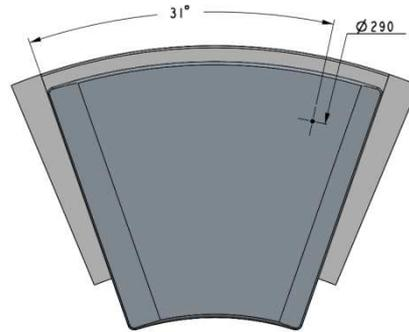
**Figure 3. PTFE faced pad showing thermocouple position**
