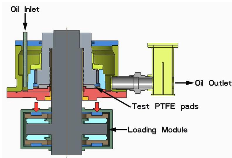
**Figure 2. Test bearing and loading arrangement**
