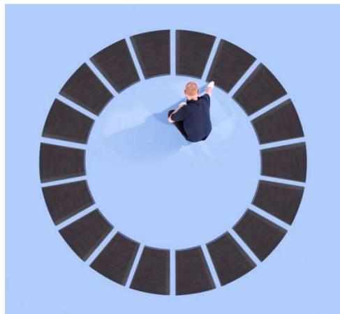
**Figure 1. Caojie thrust bearing**
