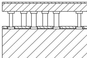
**Fig. 7 – Double Layer Thrust Pad Design**
