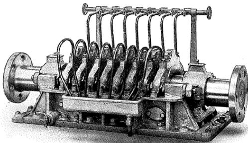
**Fig 2 – Multi-Collar Thrust Bearing**
