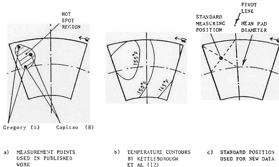
Fig. 2—Comparison of thermocouple locations and hot-spot regions
