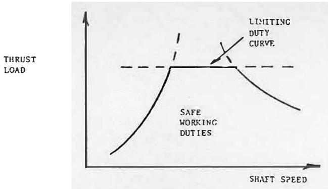
Fig. 1—Limits to thrust bearing operation
