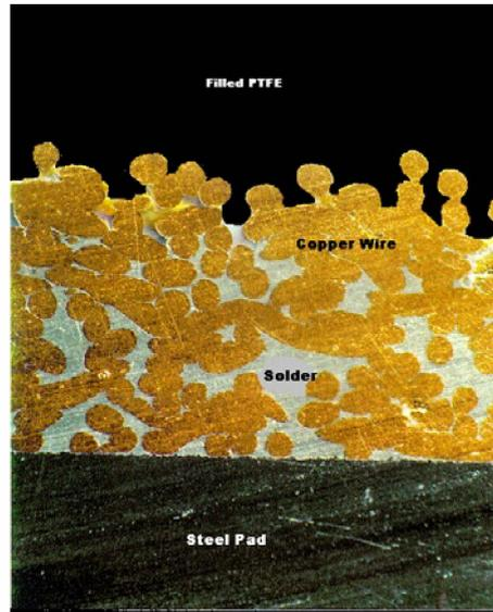
Fig. 1, Cross section through a PTFE faced pad
