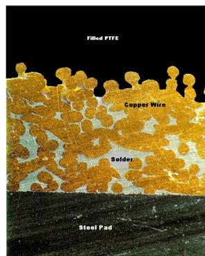
Fig.1 Cross-section through part of a PTFE faced thrust pad
