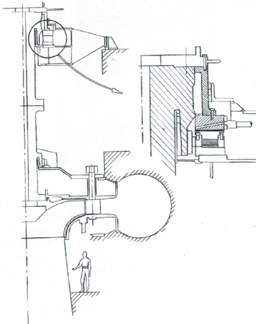
Fig. 2 Cross section through the pump turbine with reference to the thrust and guide bearing
