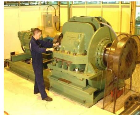
Fig. 2 Submarine thrust block test rig
