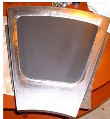
Fig.3 The PTFE faced thrust pad used in test rig
