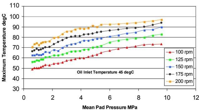
Fig. 5 Maximum thrust pad temperature v shaft speed
