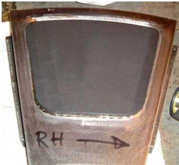
Fig. 4 A PTFE thrust pad after two months testing at 9.6MPa (1392 lbf/in<sup>2</sup>)
