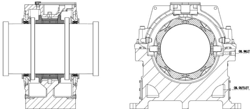
**Fig 1 – Cross Section through Test Bearing**
