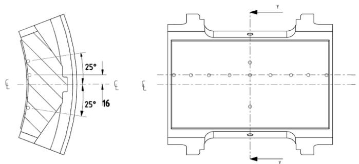
**Fig 2 – Thermocouple Positions**
