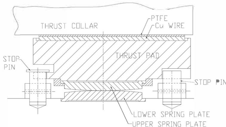
Figure 1: Thrust Pad with Spring Plate Support
