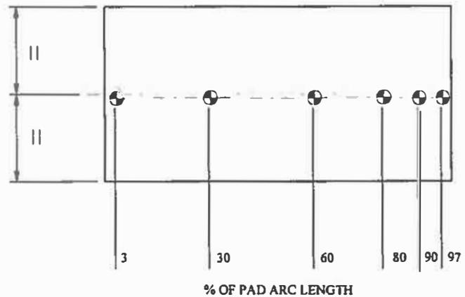
Fig. 2—Circumferential location of thermocouples relative to pad surfaces.
