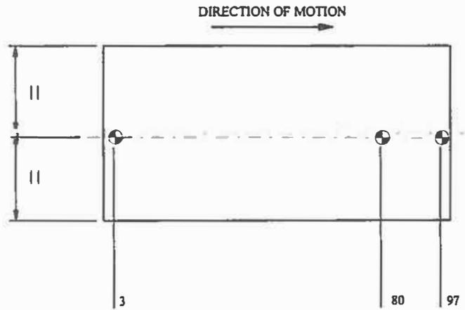
THERMOCOUPLE LOCATIONS ON PADS 1 AND 3
