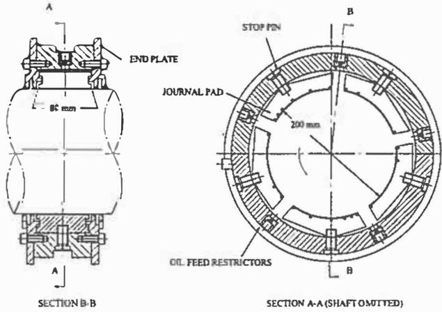
Fig. 1—Diagram of bearing used in experimental work.
