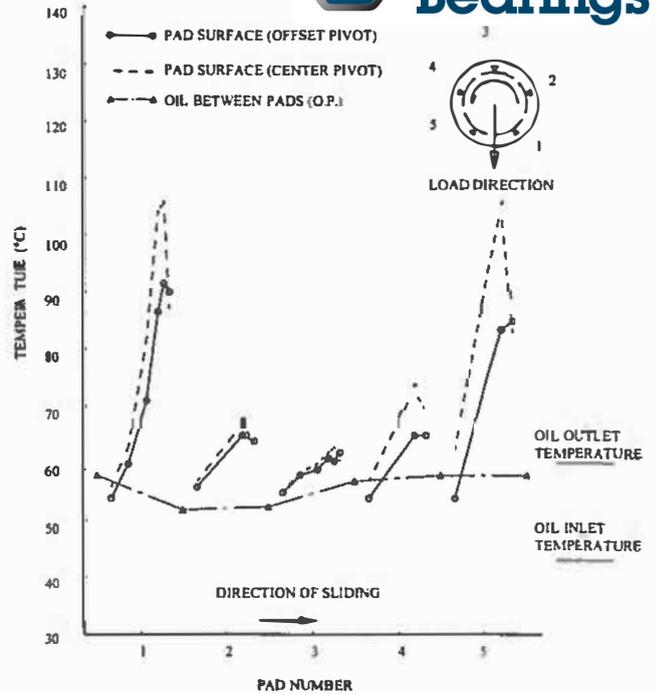
Fig. 4—Thermocouple readings obtained at 73 m/s and 2.76 MPa together with equivalent center pivot pad results from Ref. (1). Load-between-pads.
