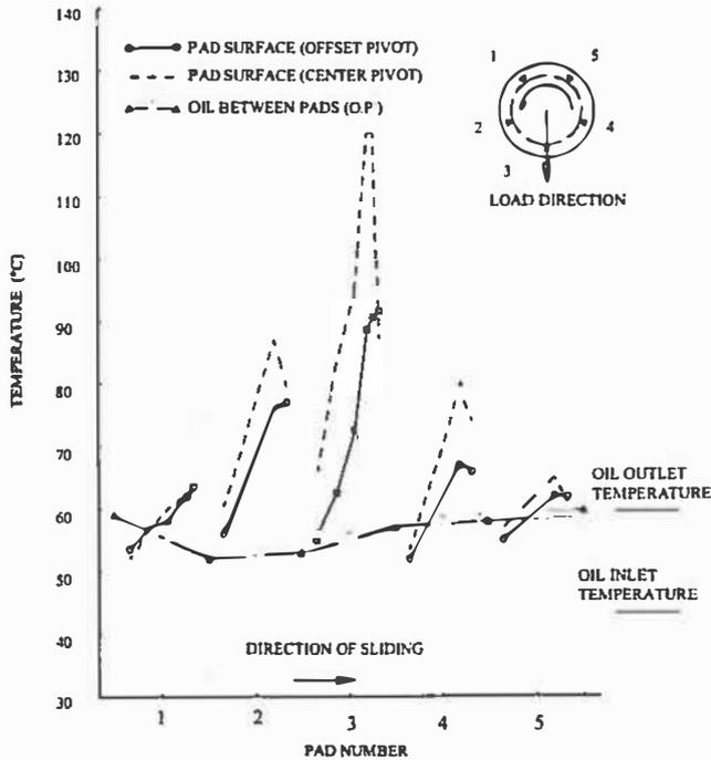
Fig. 3—Thermocouple readings obtained at 73 m/s and 2.76 MPa together with equivalent center pivot pad results from Ref. (1). Load-on-pad.
