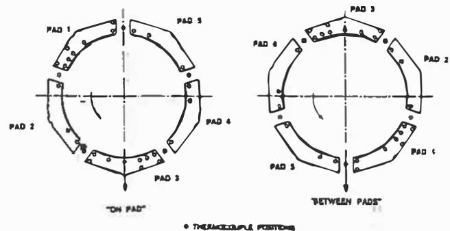
Fig. 3—Direction of applied load.
