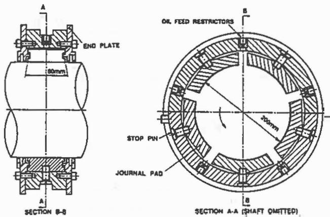
Fig. 1—Tilting pad journal bearing used in experimental work.
