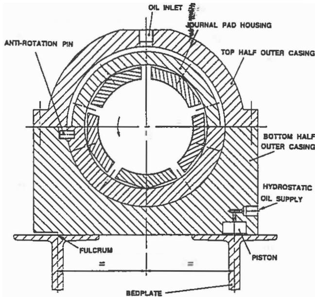
Fig. 5—Cross section of apparatus at axial midpoint of the experimental bearing.
