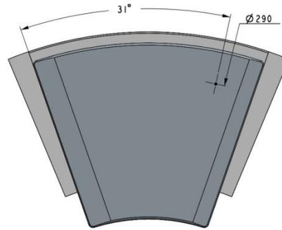
**Figure 2 – Test thrust pad showing thermocouple position**
