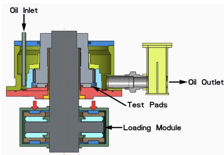
**Figure 1 – Test bearing and loading arrangement**
