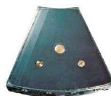
A PTFE-faced thrust pad incorporating two RTDs and HP Jacking
