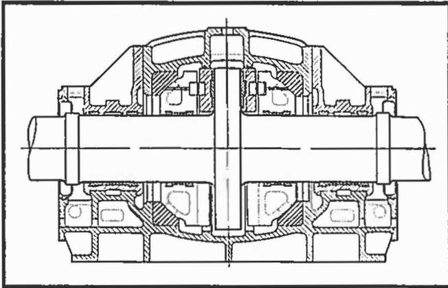
Fig 4: Typical naval thrust bearing about 1918
