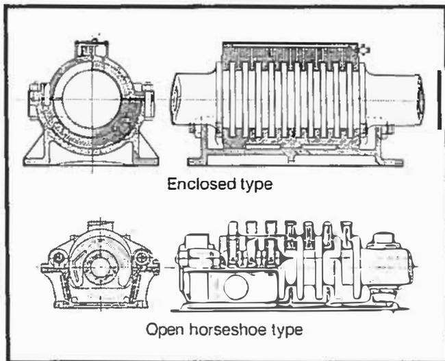
**Fig 2: Multi-collar thrust blocks**
