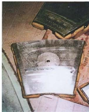
**Fig. 2, Misalignment damage to a babbitted thrust pad**
