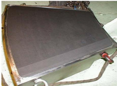
Fig. 3, The same pad as Fig. 2 converted to PTFE faced after 1500 hrs of operation.
