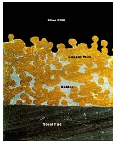
Fig. 1, Cross section through a PTFE faced pad
