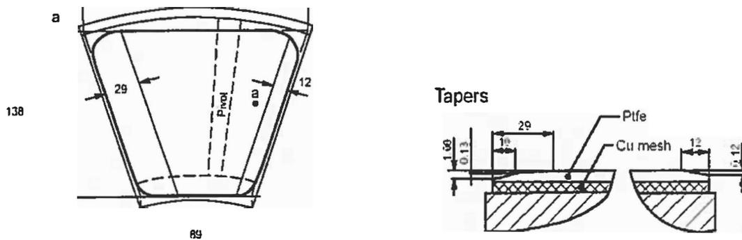
Fig 1. Pads in bearing #1
