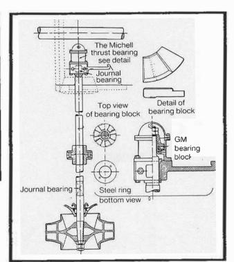
Fig 3: Michell vertical thrust bearing for a centrifugal pump installed at Cohuna on the Murray River, Victoria, 1907
