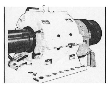
Fig 6: HMS Invincible; thrust block on test bed in maker's factory, 1979
