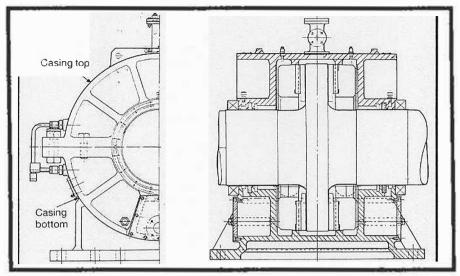
Fig 7: Concentric cylinder casing structure of a modern naval thrust bearing
