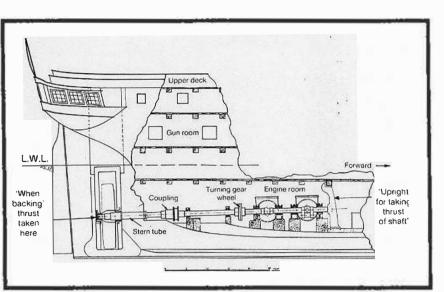
Fig 1: Screw steamship HMS *Ajax* 1848; method of receiving thrust of screw propeller in either direction
