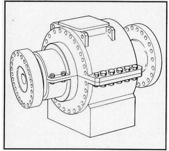
Fig 8: Bulkhead mounted thrust bearing for naval use
