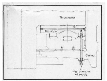
Fig 9: High pressure jacking and three piece thrust pad construction
