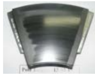
Figure 10 – PEEK pad after third temperature spike
