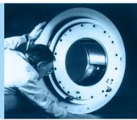
Michell Bearings offers several standard ranges of bearing internals for both thrust (Omega, Omega Equalised and Self Equalising) and radial Journal Pad Unit (JPU) applications.
