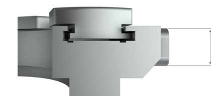
Stop key in large thrust rings
